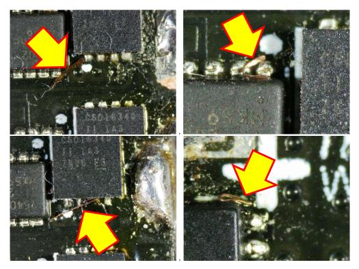
In a car that the ESC is installed the ESC should be protected from debris by placing a piece of electrical tape over the top of the board. Prior to placing the electrical tape on the ESC use a dry soft toothbrush to clean the top of the board from any potential debris that may be on the board.
